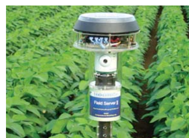
Field server to measure environmental conditions in a soybean field
