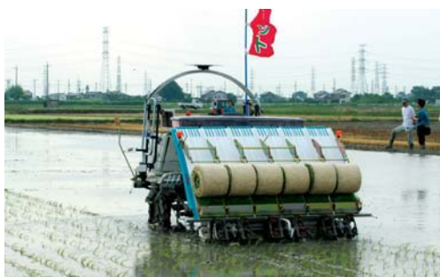
Autonomous rice transplanter using long-mat-type hydroponic seedlings
