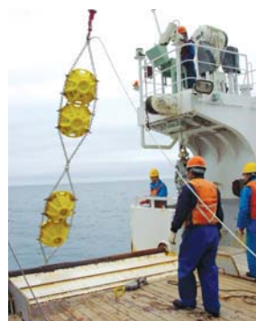
Placement of mooring systems to fix observation equipment
