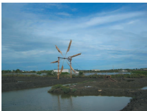
Fig.11 Purifying pond using window fans (mangrove will be planted to complete) Experimental aquaculture pond of Coastal Fishing Research Center, Kasetsart University, Thailand (Photo by Mr. Fujioka Yoshizo of IRCAS in May, 2004)
